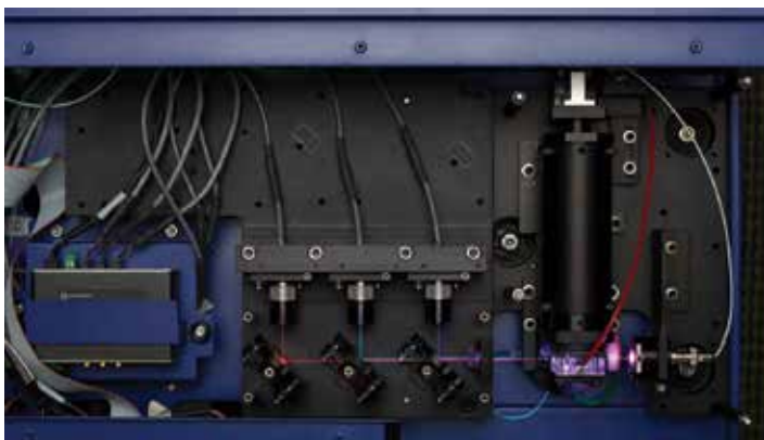
Optical deck of the BD FACSCelesta Blue-Violet-Red (BVR) laser configuration.
